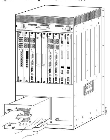
Figure 6 Removing an AC-Input Power Supply
